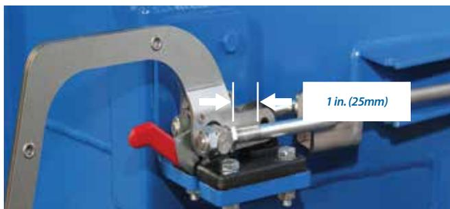
4. Begin the final adjustment by closing the Door and closing the **middle** Clamp(s) **first**. Make sure the locking lever is closed.
