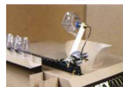
Automatic Sample Feeder The GRADEX 2000 "AutoFeed" enables staging up to seven samples for uninterrupted testing.
