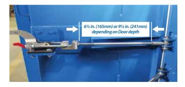
**3.** Next, adjust the U-bolt on the Clamps so there is 1 in. (25 mm) of exposed thread from the jam nut.
