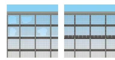
Extend the life of a worn screen frame by replacing only the tattered section of the ball support.
