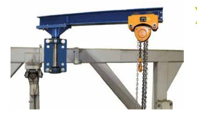
Hoist facilitates maintenance to lift drive weights, motors, and drive cartridges.
